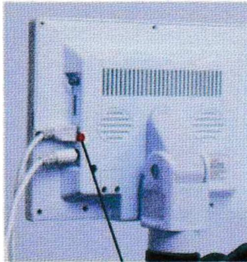
Insert the MINI USB cable into the USB port of the LCD screen.
